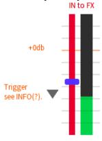
**The trigger** is set to a suggested level. Once your mic is connected and input levels set, your 'at rest' (not playing) signal level should be *below* the trigger. Ideally you should not need to move the trigger or do more than tweak levels in the interface – set it appropriately at the sound card interface. In the app window, loudest signal should be at the 0db or near.
